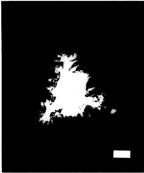
Fig. 29. Microstructure attack of Pb–Ca–Sn–Al (A903) alloy after 28 weeks (end-of-life) float corrosion in VRLA battery held at +60 °C. Localized penetration with bulk oxidation. Triangular grid member (reference bar 440 \mu\text{m} ).
