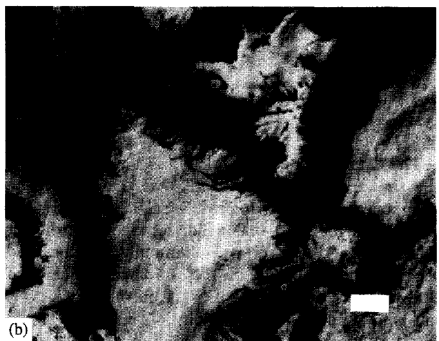
Fig. 33. (a)(b) Details of microstructure attack of Pb–Ca–Sn–Al (A707) alloy after 54 weeks (end-of-life) float corrosion in VRLA battery held at +60 °C. Narrow penetration along grain boundaries followed by slow attack of bulk of grain with a comb-like corrosion front (reference bar 24 μm).
